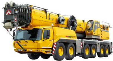
GMK6300L-1 CAPACITY 300 t MAIN BOOM 80 m MAX TIP HEIGHT 120 m
